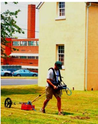
*Archaeologist, Shawn Patch uses GSSI's ground penetrating radar to identify features consistent with previous buildings, wells, and privies at a former plantation built in 1795 in Greensboro, North Carolina. The GPR data was used to guide excavations at a summer field school.*
